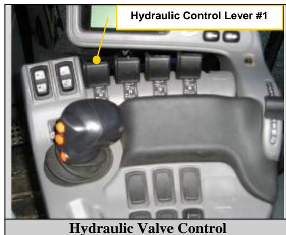
8. Start the tractor and move the hydraulic control lever all the way forward to FLOAT position.
