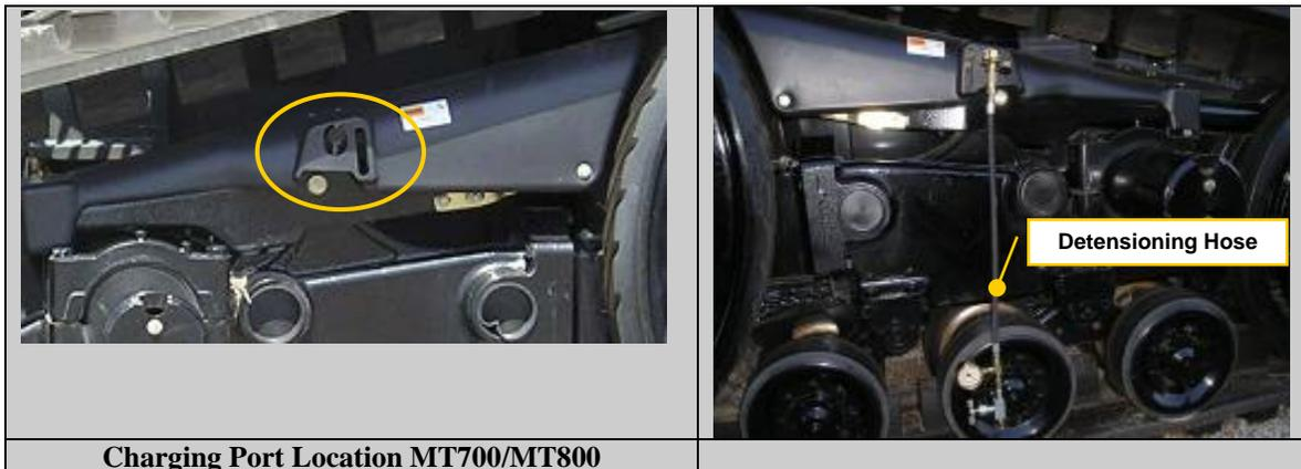
6. Connect the opposite end of the detensioning hose to the lower port on the hydraulic valve bank at the rear of the machine.
