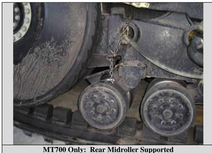
Note: removal of the track will require the use of either a forklift or a boom truck, as the tracks weigh between 800 and 2100 lbs each. Use care when removing tracks or injury could result.
